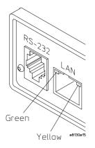
The yellow LED, on the right side of the connector, indicates LAN activity (receive or transmit).
