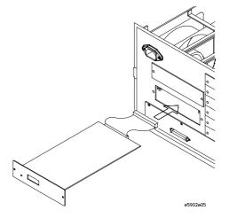
6 Connect the cable and re-install the screws.
