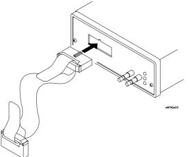
Connecting the Emulation Probe to Your Target System **To connect the emulation probe to the target system**
