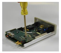
**5** Carefully lift the target board adapter from the main circuit board.
