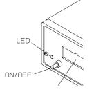
The green LED, to the left of the power switch, is lit when the emulation probe is connected to a power source and the power switch is on.
